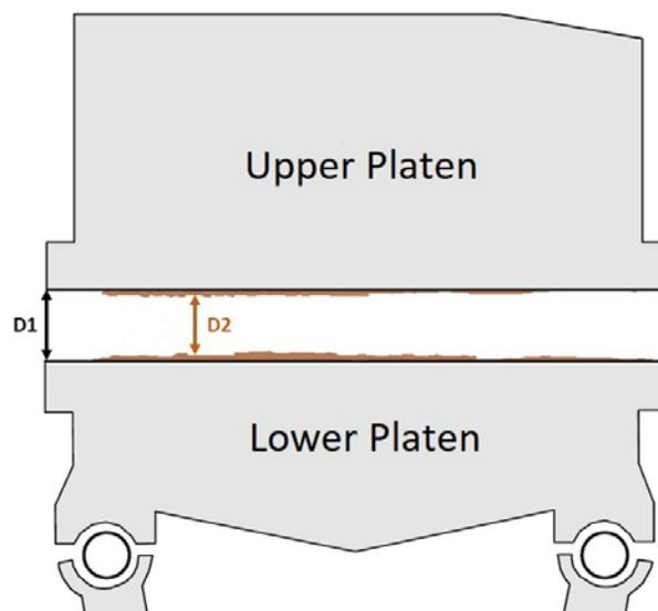
Unevenness because of rust and dirt also occurs on the plates of the upper chase and the lower counter die-cutting bed (Fig. 2 - 5).
