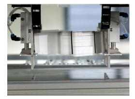
The sheets are then transferred to a conveyor belt using an automatic gripper.
